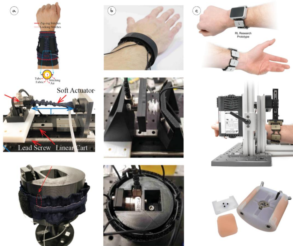
Figure 39. Wearable haptic devices and characterization methods: (a) Column showing PneuSleeve device worn on forearm with labeled components, its actuation mechanism with lead screw and linear part, and the complete prototype; (b) Column displaying Bellowband wrist-worn device, its force measurement setup, and internal component view with embedded sensor; (c) Column presenting Tasbi wrist-worn research prototype, its force characterization setup using ATI Nano 17 sensor, and the device components.
