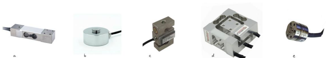
Figure 23. Various types of load cells: (a) beam load cell, typically used for precision weighing; (b) bottom load cell, designed for compression force measurements; (c) S-type load cell for both tension and compression; (d) 3-axis load cell for multi-directional force measurement; and (e) force-and-torque load cell measuring both rotational and linear loads.
